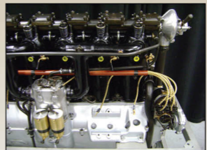
Water jacketed intake manifold and carburetor detail. A mount for the generator (643) can be seen at right but the actual generator was very rarely installed in fighter aircraft unless used to power an electrically heated flight suit or wireless transmitter.
