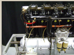
Water jacketed intake manifold and carburetor detail. A mount for the generator (643) can be seen at right but the actual generator was very rarely installed in fighter aircraft unless used to power an electrically heated flight suit or wireless transmitter.
