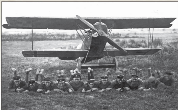
This unidentified mid production Fokker D.VII (OAW) was reportedly with Jasta 41 when this photo was taken. Note the far outboard position of the post June 1918 'even arm' balkenkreuz which is an identifying feature introduced towards the end of the 2nd OAW production batch (numbers 4000/18 to 4199/18), all 3rd production batch aircraft (numbers 4000/18 to 4199/18) and the initial 40 or so machines from the 4th production batch (numbers 6300/18 to 6649/18).
