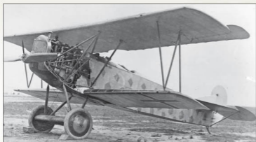
This unidentified and unarmed late production OAW built Fokker D.VII was photographed after the armistice and features a washed out 5 colour lozenge covered fuselage (probably with a 'glaze coat of brown tinted dope), double rudder control horns and radiator with offset filler cap. Note the protective 'stacking' pads on the leading edge of the wings.
